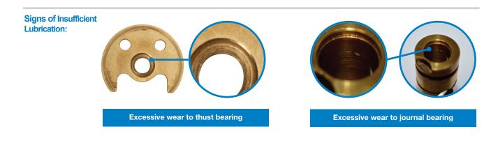
Preventing turbo failure caused by Insufficient Lubrication:
